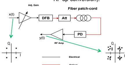
DFB: Distributed Feedback laser; PD: Photodiode; Att optical attenuator.
