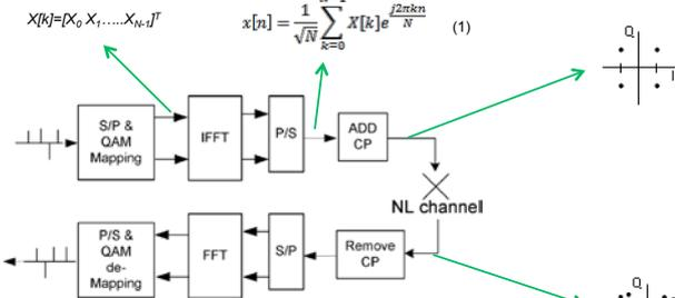
Simplified diagram of OFDM transmitter and receiver. S/P is serial-to-parallel conversion, P/S is parallel-to-serial conversion, CP is cyclic prefix. Represents model used in simulations.
