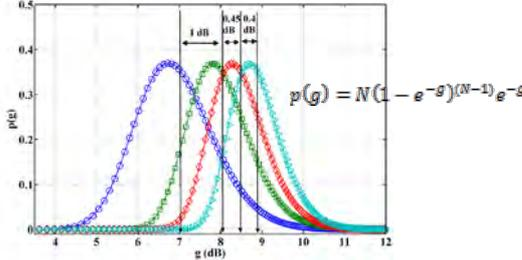
PDF of statistical PAPR for different IFFT sizes. The annotations correspond to differences between the medians for different IFFT sizes.
