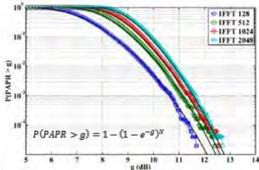
CCDF of PAPR: solid traces are analytical results, points are simulation results from Matlab.
